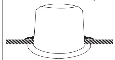
Snap it into place on the ceiling and gently leave the hooks to fit the speaker in. Do not leave gaps on the grill side.
