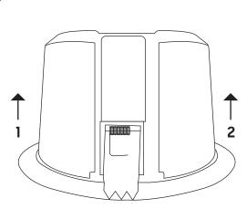
Hold the front side of the speaker with your hand, pull the 1st side up and then the 2nd side up to open the cover.
