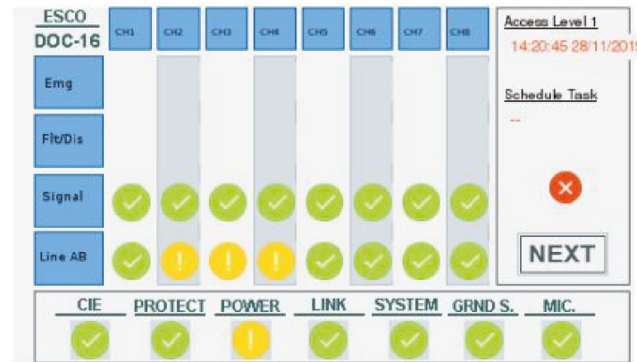
Figure 3 - Amplifier and zone monitoring screen (DOC16 example)
