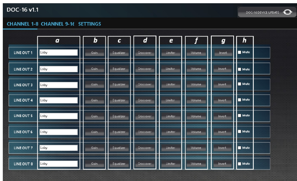
Figure 20 – DOC16 output controls
