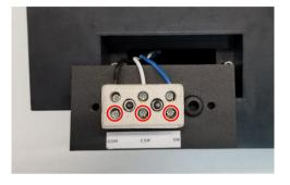
Loosen the screws seen in the above figure which are going to be used for the application. For 2.5W, use COM and 2.5W; for 5W, use COM and 5W.
