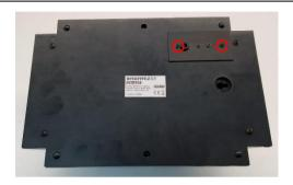
Open the small lid, behind of the speaker, by unscrewing the two marked places in the above figure.
